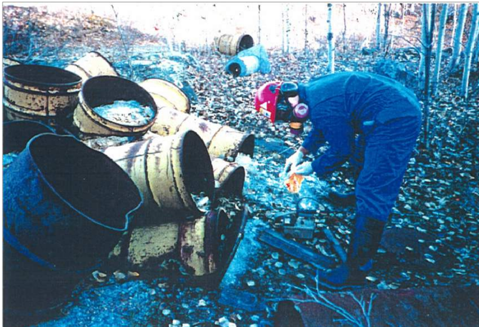
Sampling ‘hot’ barrels (PWGSC)
